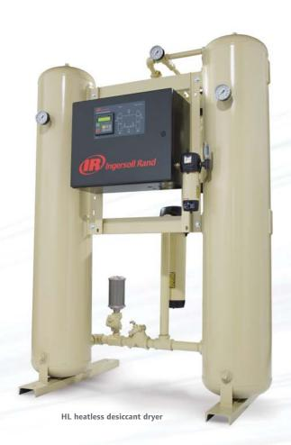
Available in flows ranging from 2.5 nm<sup>3</sup>/min. (90 scfm) to 141.6 nm<sup>3</sup>/min. (5,000 scfm), Ingersoll Rand HL heatless desiccant dryers are designed to ensure a constant -40°C (-40°F) or optionally -70°C (-100°F) pressure dew point, virtually eliminating costly interruption of production due to moisture. Clean air is further assured by use of strategically placed filters: a pre-filter to remove oil and contaminants in air
