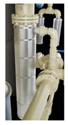
High efficiency heater reduces air needed to regenerate desiccant.
